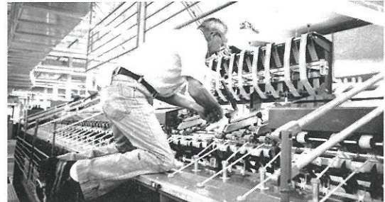
Grover Laye from Plant No. 22 is shown fixing a Zinser Roving Frame.
