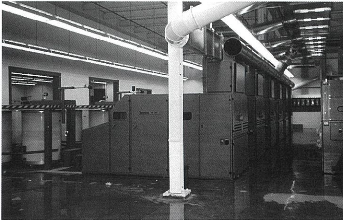
Trutzschler DK803 High Production Card: This machinery enables increased production, while maintaining quality. These cards feature the integration of the card and the tuft feeder. This guarantees an even web feeding into the card, improvement of web evenness, simplified maintenance, a reduction in operation costs, and the elimination of possible operating and adjusting errors.
